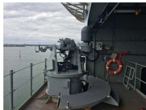
Photo: Canberra's force protection weapons system includes a 25 mm M242 Bushmaster chain gun and a coaxially mounted M240 7.62mm machine gun.
